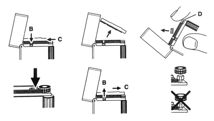
Put the flint into the channel against the flintwheel. Replace the slider «C» pushing it forward with your index finger. The pin «B» should now go back to its initial position.
